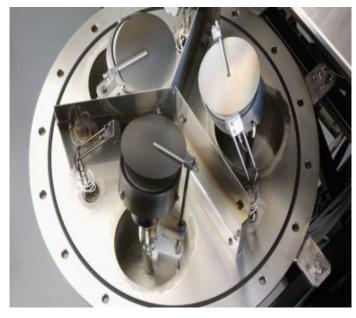
In sputtering atoms are ejected from a solid target due to bombardment by energetic particles in plasma status. Deposits thin film of metals such as Al and Au and dielectrics such as ITO (Indium Tin oxide) and ZnO.
