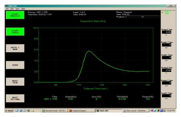
4 – If the power rose at a good speed and then the rate overshot more than 50-60% and then came back down at a good speed then your I value is most likely very close to being right. You then have to increase the P value to drive the system both up and down faster to reduce the overshoot.
