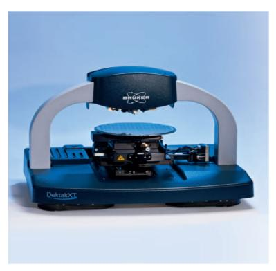
Surface profiler measures small surface variations in vertical stylus displacement as a function of position. This profiler can measure small vertical features ranging in height from 10 nm to 1 mm.
