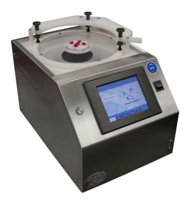
Spinner spin-coats very uniform and thin layer of photoresist and e-beam resist on substrate even thinner than 100 nm. It can hold 5" wafer. Maximum spin speed is 12,000/minute.
