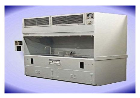
Fume hood for processing such as cleaning samples, wet chemical etching, developing of pattern, lift off after deposition, metal plating,
