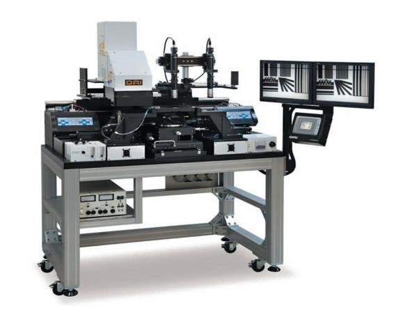
This mask aligner can transfer the pattern on the optical mask on the substrate with spin coated photoresist. It can hold to  $5 \times 5$  " mask. The backside or front side alignment is available.
