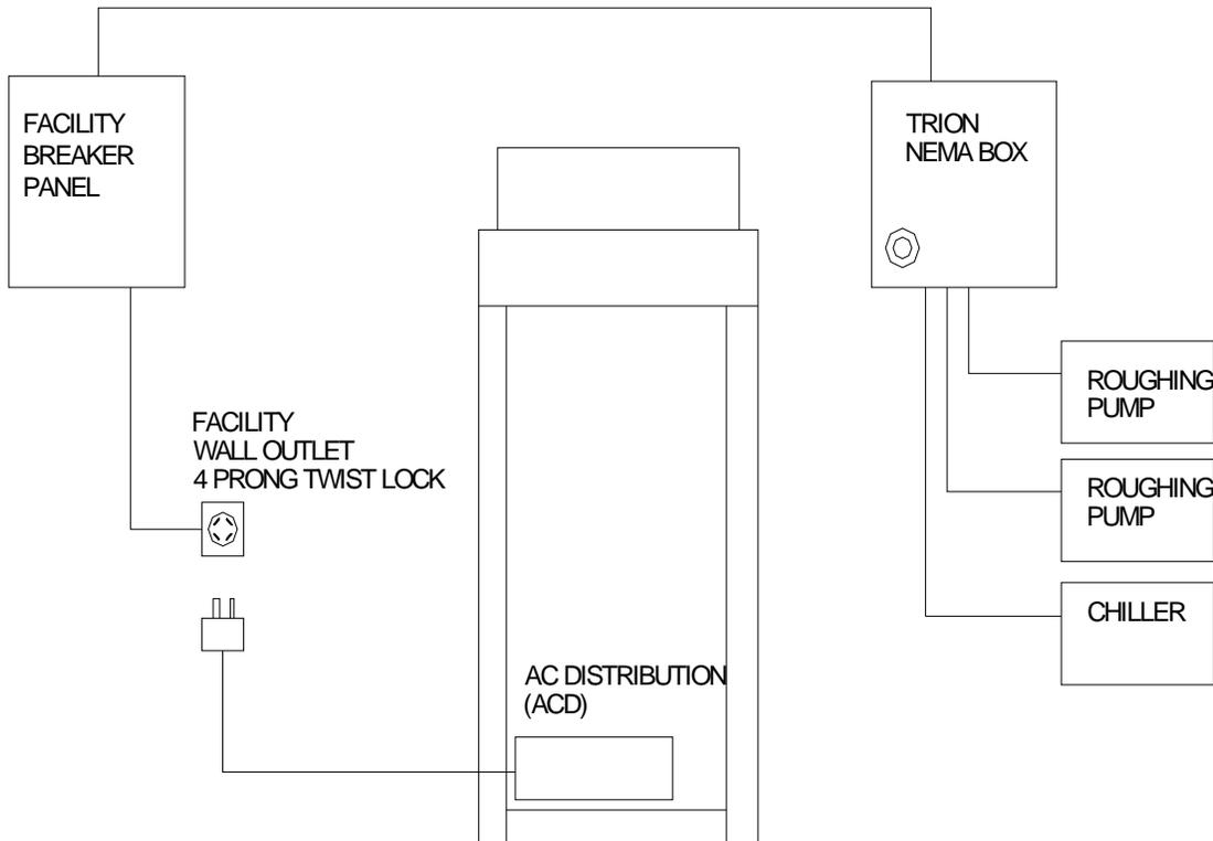
**Figure 7** Main Electrical Distribution Diagram
