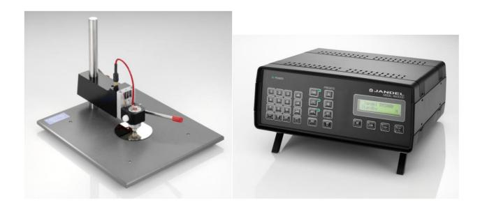
4-point probes measurement system is an electrical impedance measuring technique that uses separate pairs of current-carrying and voltage-sensing electrodes to make more accurate measurements than traditional two-terminal method. 4-point probes are used to measure resistivity of bare silicon wafer and sheet resistance of thin films.
