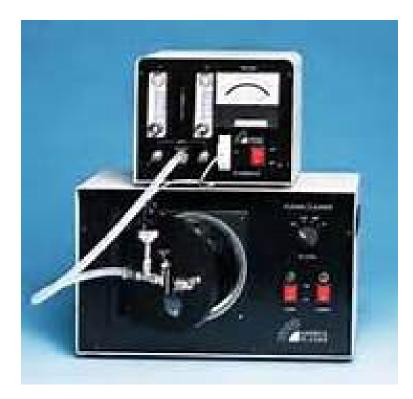
The plasma cleaner is to be used to remove impurities and contaminants from surfaces through the use of energetic plasma created from gaseous species. Gases such as argon and oxygen, as well as mixtures such as air and hydrogen/nitrogen are used.
