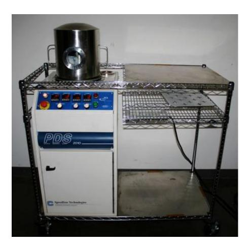
SCS lapcoater system performs reliable and repeatable application of parylene conformal coating and applies parylene coatings to components such as circuit boards, sensors, wafers, medical devices, MEMS for research and development. This tool deposits parylene thickness from hundreds of angstroms to several mils, a typical thickness is in the microns range.
