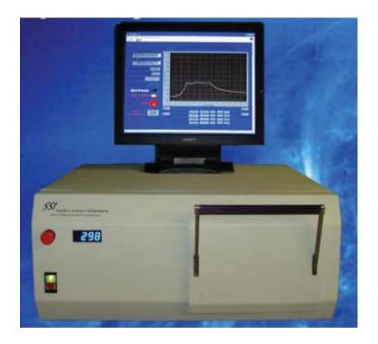
RTA can be used in order to activate dopants, change film-to-film or film-to-wafer substrate interfaces, change states of grown films, repair damage from ion implantation, move dopants or drive dopants from one film into another or from a film into the wafer substrate, form ohmic contact metallization for HBT, MESFET, HEMT, Solar Cell, LED, Sensors. It can be reached to maximum temperature of 1200°C in seconds.
