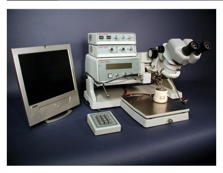
Wire bonder makes interconnections between an integrated circuit (IC) or other semiconductor device and its packaging during semiconductor device fabrication. It is used to assemble the vast majority of semiconductor packages.
